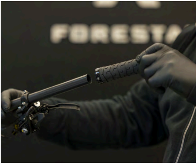
Step 1. Slide the lock-on grip to the handlebar.
