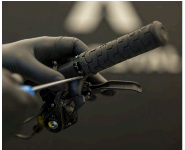
Step 2. Tighten the lock-on grip to 2.5 – 4 Nm using a 3mm hex key.
